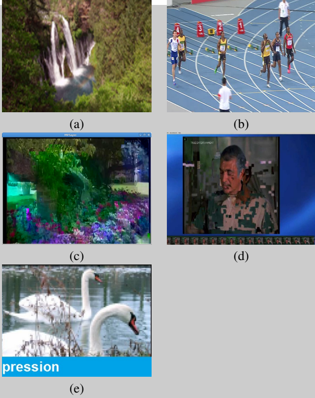
Fig. 1. The publicly available web crawled sample images with bad quality due to (a) up-scaling, (b) combing/interlacing, (c) H.264 hits, (d) MPEG-2 hits and (e) compression.
