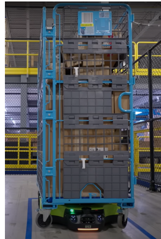
Fig. 3. Proteus robot lifting a cart
