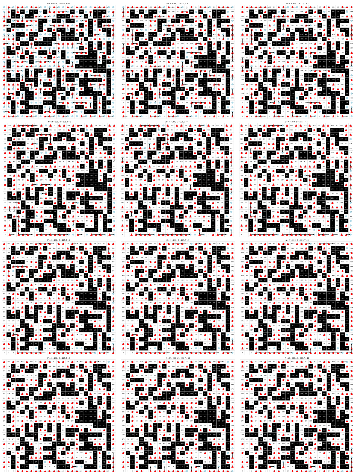
Figure 9. A 25 \times 25 grid with \{200\} robots \blacktriangle , \{200\} targets \bullet , and \{225\} obstacles. Every cell is either a robot, a target, or an obstacle. The robot trajectories come from the min-cost (optimal) transport obtained from \mathbf{P1} over T = 12 .
