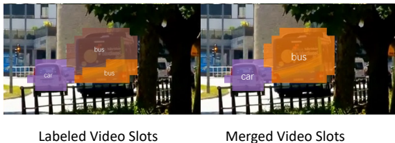
Figure 4. Joint optimization. The image on the left shows one frame of video slots with target names, the image on the right shows the result from merging. The two slots for the bus are merged thus better localizing the object, while they don’t further merge with the slot for car since they share different semantics.
