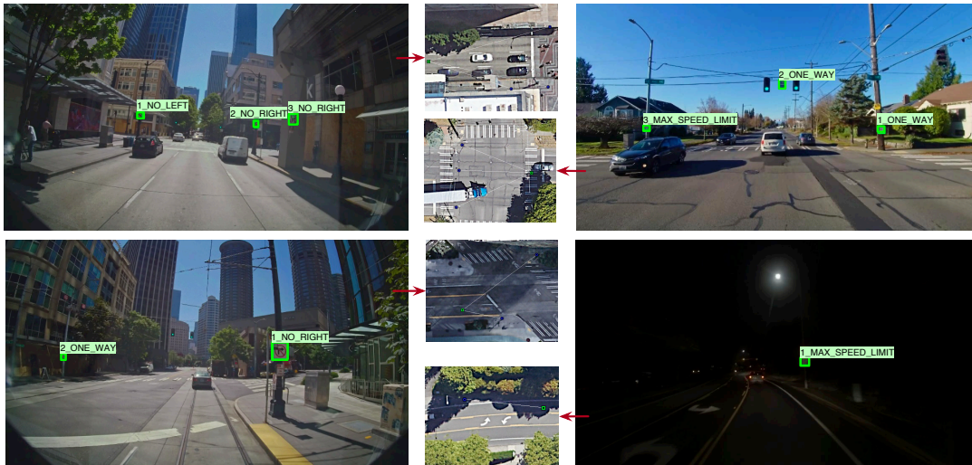
Figure 5: Qualitative localization accuracy of traffic signs. Traffic sign bounding boxes at an image and corresponding geo-referencing locations are shown on the map pointed by the arrow. On the map view, we show the frame location with a green square and sign locations with blue circles. The map view also shows white lines between a frame and localized signs. The right-bottom image shows a night example.
