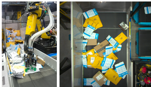
Fig. 1: An example of a Robot induction (Robin) workcell. Robin performs automated package singulation by picking packages from unstructured piles on conveyors and transferring them to mobile robots.
