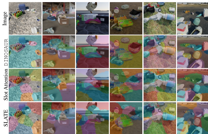
Figure 20: Masks on MOVi-E using 11 instead of 24 slots (quantitative results in Table 13). Our method uses a ViT-B/8 encoder and the MLP decoder.
