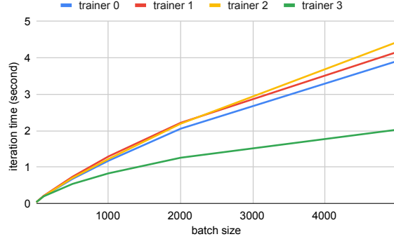
Figure 3. The iteration time when training a GraphSAGE model with four trainers using DistDGL. The running time varies across trainers indicating workload imbalance. Larger batch size increases running time but not linearly.
