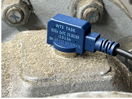
Figure 3. An accelerometer sensor attached to equipment
