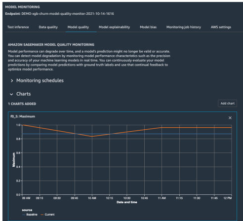
Figure 5: Model Quality tab in SageMaker Studio showing of Model Monitor Model Quality calculation of the F0.5 score for a binary classification model
