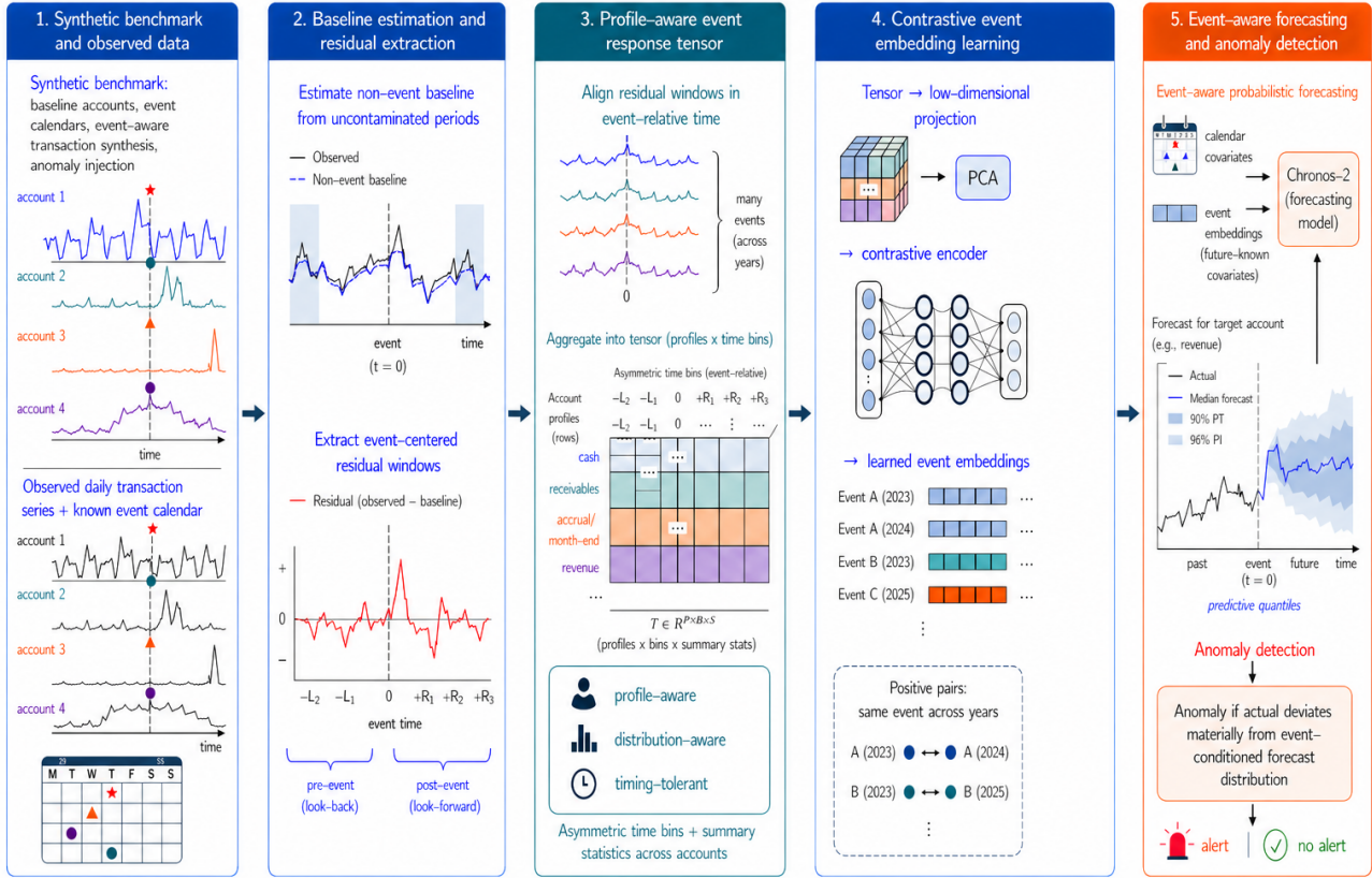
Figure 1. Overview of the pipeline. Event-centered residual responses are extracted from observed series, aggregated into profile-aware event-response tensors, transformed into learned event covariates, and supplied to a pretrained forecasting model for anomaly detection.
