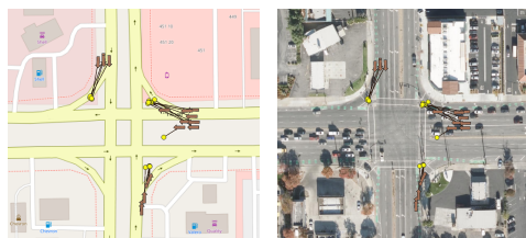
Fig. 7: Detections at complex intersections including slip/via lane involves decision to first identify and next target multiple intersection nodes are rejected by auto-reviewer model. Legend: yellow circles as detection locations, brown arrow as vehicle location and heading, respectively.
