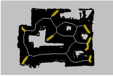
Fig. 4. Computed skeleton, with problematic spurs highlighted in yellow. These spurs enter narrow spaces or corners but do not represent typical walking paths, so they need to be removed from the skeleton to avoid erroneously marking those areas as blocking .
