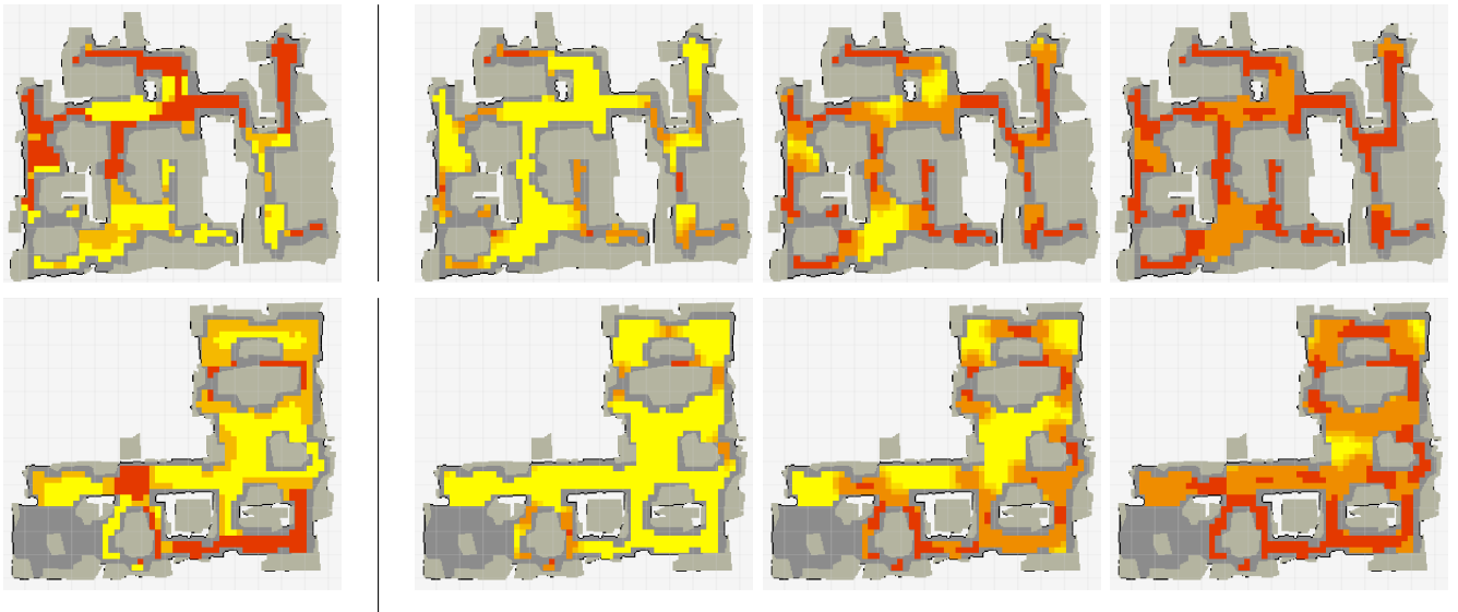
Fig. 7. Examples of two floorplans. Left: User-annotated preference map. Center to right: Availability maps generated for dH values of 25cm, 45cm, and 65cm. Red represents bad parking spots and yellow represents good. By inspection, the 45cm map gives the closest fit to the user-annotated map.
