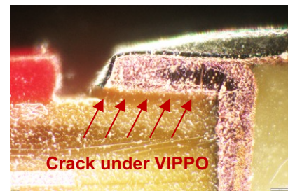
Figure 4. Optical image of VIPPO pad crater cross-section
