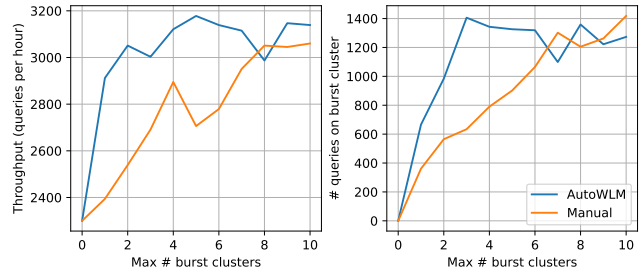
Figure 5: Behavior of Auto-WLM concurrency scaling compared to a manual baseline for TPC-DS 100G. The x-axis represents the maximum number of concurrent clusters Auto-WLM is allowed to create (with zero meaning that horizontal concurrency scaling is disabled). The left plot shows the throughput of the cluster, which increases as the number of allowed concurrency scaling clusters increases. The right plot shows the total number of queries assigned to concurrency scaling clusters at each configuration.
