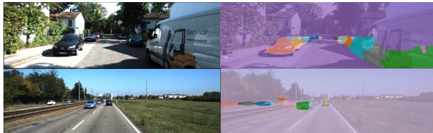
Figure 7. DINOSAUR grouping results on KITTI. We observe that the masks are imprecise, especially for objects that are far away.
