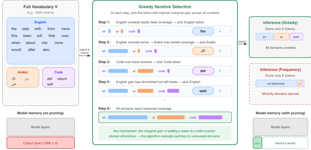
Figure 1: Mechanism of greedy vocabulary selection. Left: the full vocabulary holds a large English cluster beside smaller minority-domain clusters (Arabic, code), and the output layer dominates model memory. Center: greedy picks the token of highest marginal gain across calibration contexts. As a domain becomes well covered its gains diminish, so the algorithm switches to the least-covered domain, balancing coverage after K steps. Right: at inference only K tokens are scored.
