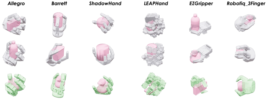
Fig. 3: Qualitative results on unseen validation object. The first two rows show hands trained with full grasp annotations (rendered in gray); the third row shows annotation-free hands trained solely through the morphology prior path (rendered in green).
