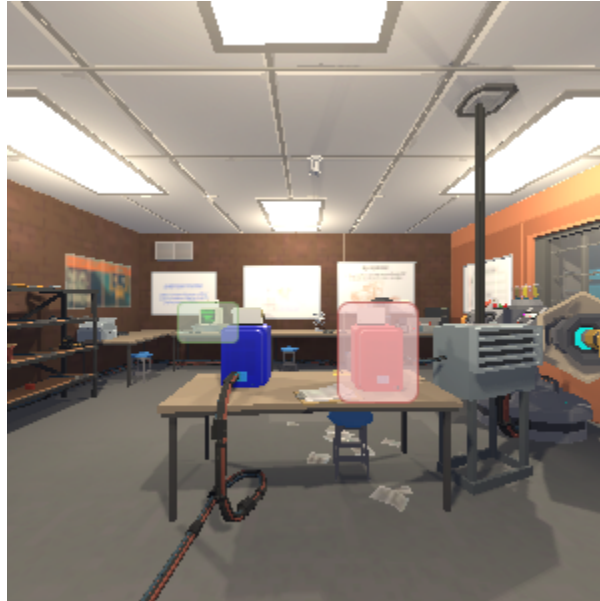
Figure 3: Grounding Failure An example of where our system would fail would be if the user asked “Turn on the computer furthest away from you” when presented with this situation. Our current system would predict [GoTo: Computer, Toggle: Computer] and our grounding module would choose the largest mask it sees which would be the computer highlighted in red, instead of the computer highlighted in green which the user intended to interact with.
