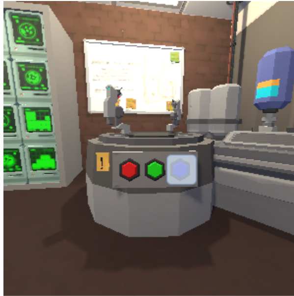
Figure 4: Grounding Success An example of where our system would succeed would be if the user asked “Press the blue button” when presented with this situation. Our current system would predict [Toggle: Button] and indicate that we are looking for blue object. The color detector would filter down all vision predictions not predicted as blue and our grounding strategy would choose the mask for the button highlighted in blue.
