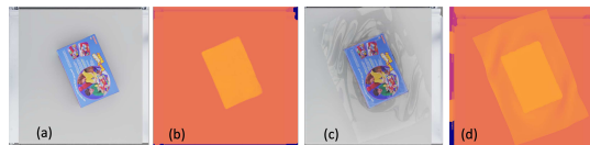
Fig. 4: (a) RGB without translucent barriers, (b) Depth image without barrier (c) RGB with translucent barriers, (d) Depth with the translucent barrier. In addition to these, this dataset also contains RGB from a stereo pair, the intrinsics and the semantic segmentation
