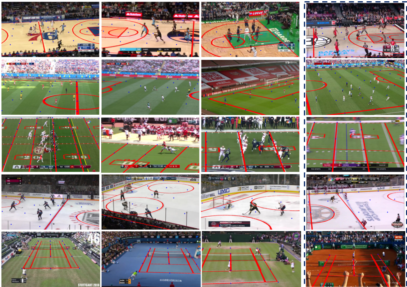
Figure 6. Qualitative results of our approach ( ours – all ) for challenging examples from five different sports in our SportsFields data. Four examples of each sport are visualized with sport field lines (red) and keypoints (blue) overlaid on the image. The last column shows one failure example for each sport. More qualitative results are presented in supplementary materials.
