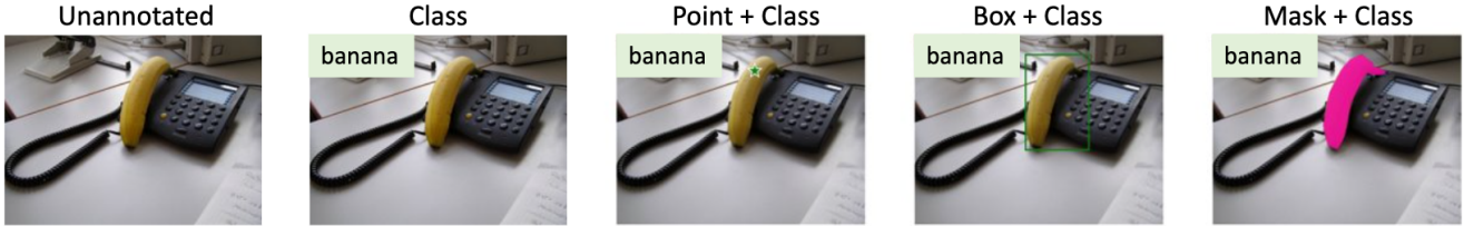
Figure 3. This figure displays the types of per-instance annotations considered in this work. The mask + class annotation represents the strongest form of annotation, and is required for fully supervised instance segmentation.
