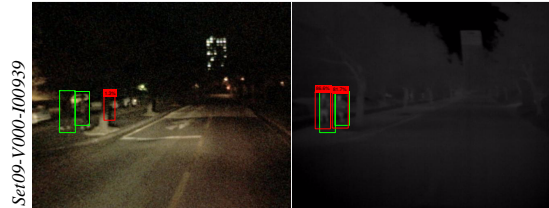
Fig. 1: During night time, pedestrians detections (red) are more accurate in the thermal image (right) than the color image (left). Ground truth boxes are shown in green.
