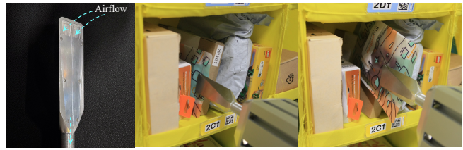
Fig. 11. Side-way suction on a blade-style tool. We explored pick poses and motion strategies to utilize the new modality to pick narrow items using their side surfaces.
