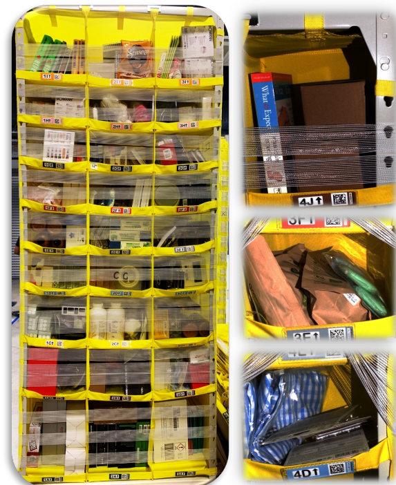
Fig. 1. Example of a fabric pod (left) and a number of its individual bins (right) containing a range of items. Elastic bands and bin lips at the bottom of the bins prevent items from falling out when the pod is transported to a picking station by a mobile robot. The metallic frame holds the fabric and obstructs items behind. Individual items are often obstructed or stacked. The images of the two bins (bottom-right) are captured while the band separation system, a subsystem of our overall autonomous pick solution, is holding the elastic bands during the extraction process.
