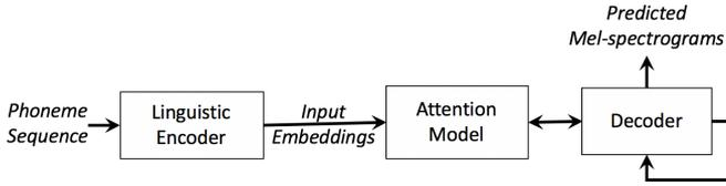
Figure 1: Schematic diagram of a seq2seq Neural TTS
