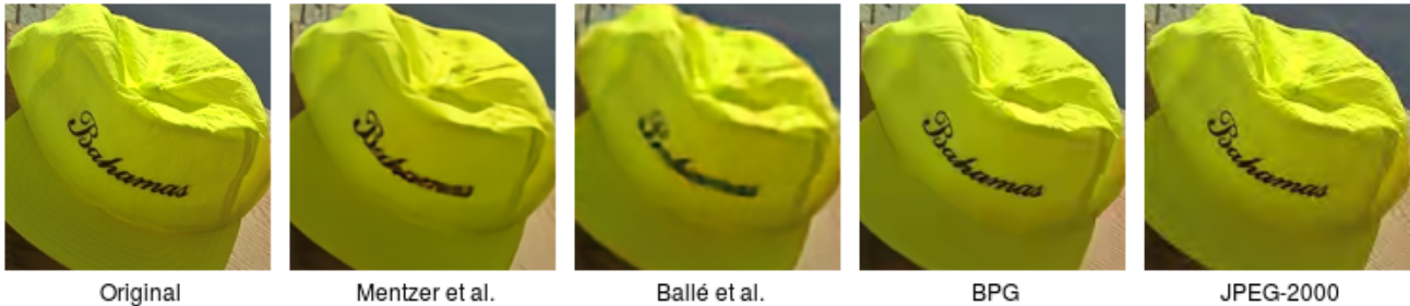
Figure 1: An example from the Kodak dataset [12]. In order of MS-SSIM values: Mentzer et al. [26] > Ballé et al. [3] > BPG [5] > JPEG-2000 [37]. However, the order of performance based on 5 human evaluations is: BPG [5] > Mentzer et al. [26] > JPEG-2000 [37] > Ballé et al. [3]. Visually the foreground and text in BPG is clearly better in quality.
