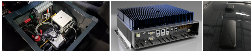
Figure 1: Experimental setup. From the left: reference ground truth system, in-vehicle computer with precision GNSS module, low-cost antenna on the roof.
