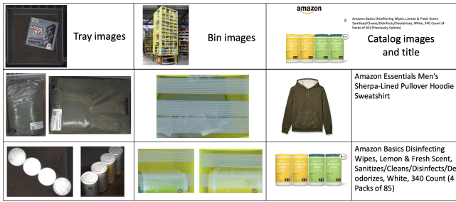
Fig. 2. Examples of the four different reference sources used for object identification. The Tray and Bin images are acquired during fulfillment operations and are representative of packaged state of objects while Catalog images and text are descriptions of the object typically used in an online catalog or webpage.
