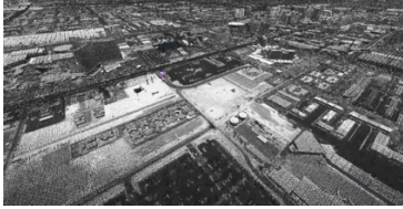
Figure 1: Visualization of USGS 3DEP LiDAR data in Las Vegas, hosted via Entwine Point Tiles format [10].
