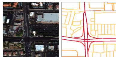
Figure 6: Visualization of multi-class road mask. Left: RGB image tile. Right: road mask with color coding in which yellow-to-red colormap represents speed values from low to high speed (0-65 mph).
