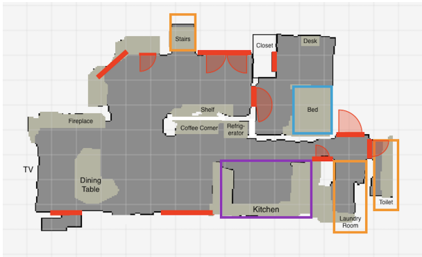
Fig. 6. An example 2D-L map. Contextual information is explicitly identified to help annotators provide an informed rating of social appropriateness for a given potential robot parking position. Light brown areas represent clutter or furniture, red arcs or line segments indicate doors, colored boxes indicate kitchen, other rooms, or beds, and the remainder of features are labeled with text. 1-meter grid lines provide scale reference.
