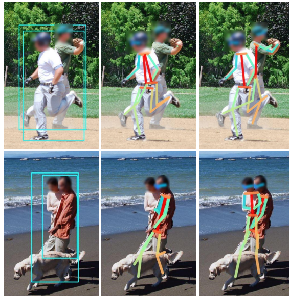
Figure 1: 2D pose estimation networks often fail in presence of heavy occlusion. (Left) Bounding boxes corresponding to two persons. (Middle) For both bounding boxes, HRNet predicts the pose for the front person and misses the occluded person. (Right) MIPNet allows multiple instances for each bounding box and recovers the pose of the occluded person.
