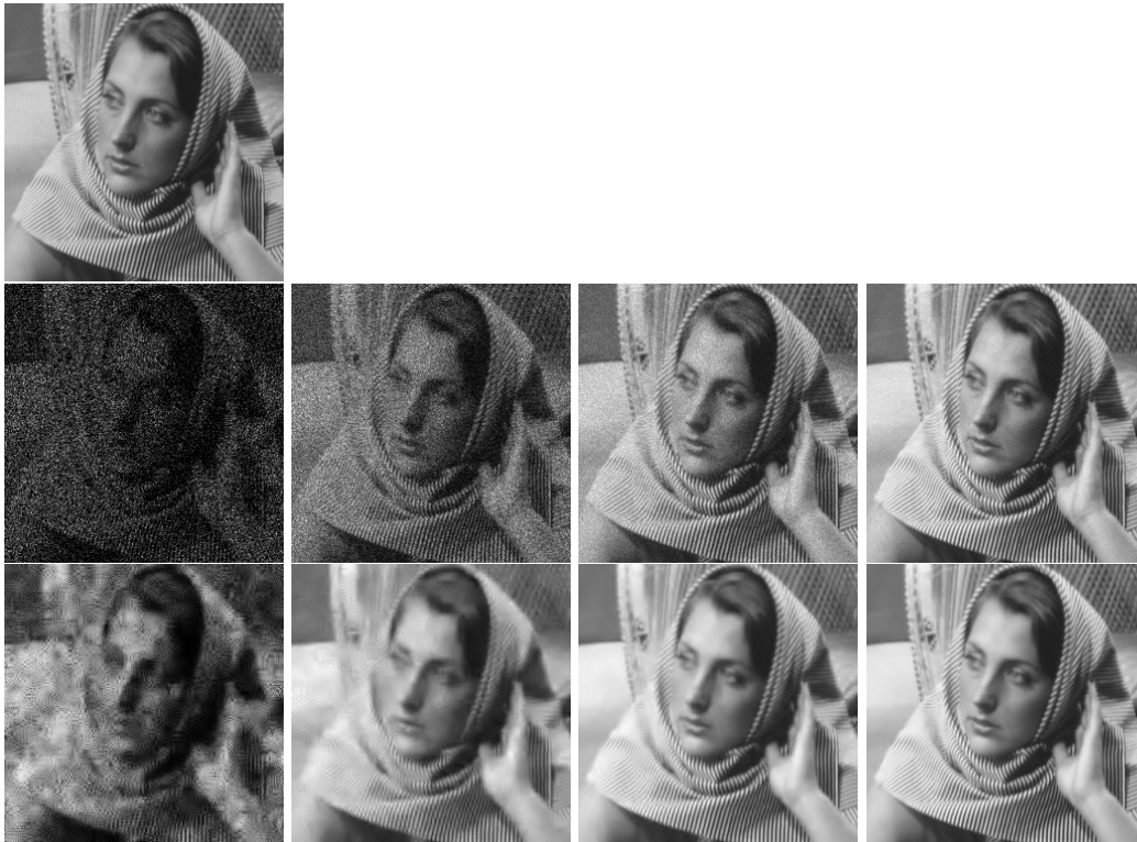
Figure 4: Topmost row: original Barbara image; Second row: noisy images generated from underlying clean images with intensity 10^5, 10^6, 10^7, 10^8 respectively; Third row: denoised images corresponding to their noisy versions from the row above (RMSE values 0.4, 0.128, 0.0597, 0.0264 respectively). See Sec. 3.3 for more details.
