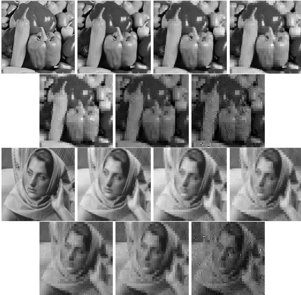
Figure 3: Left to right, top to bottom in each group: Original image, followed by image reconstruction results using VST2-AUTO for 8 \times 8 image patches with N = 45 measurements per patch, for six different image intensity levels I \in \{10^9, 10^8, 5 \times 10^7, 10^7, 5 \times 10^6, 10^6\} . Refer to Sec. 3.2 for more details, and to Table 3.2 for RRMSE values.
