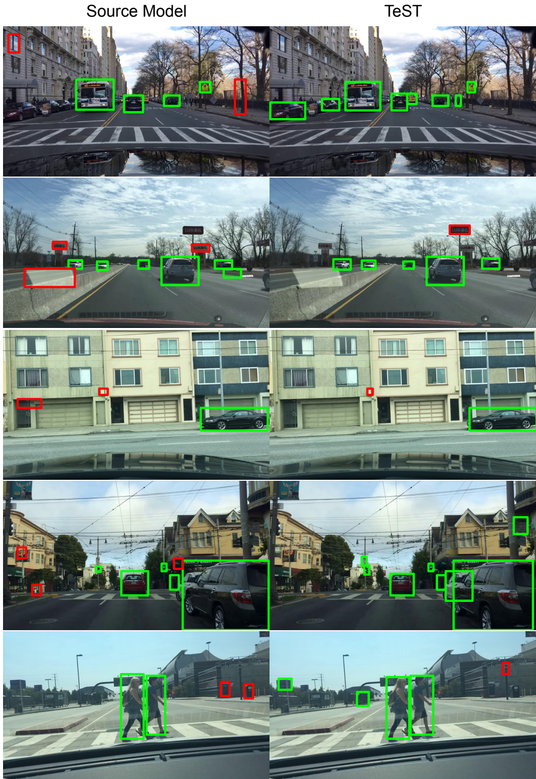
Figure 11: Qualitative results from BDD100k with a Deformable DeTR Object Detector [70]. True positives are shown in green rectangles and False positives are shown in red rectangles. We note that: all images are chosen at random without any cherry-picking. We see that the models trained with TeST have fewer false-positives and more true-positives, which strongly suggests that TeST is able to improve the final object detector on the novel dataset. We see that the models trained with TeST have fewer false-positives and more true-positives, which strongly suggests that TeST is able to improve the final object detector on the novel dataset.
