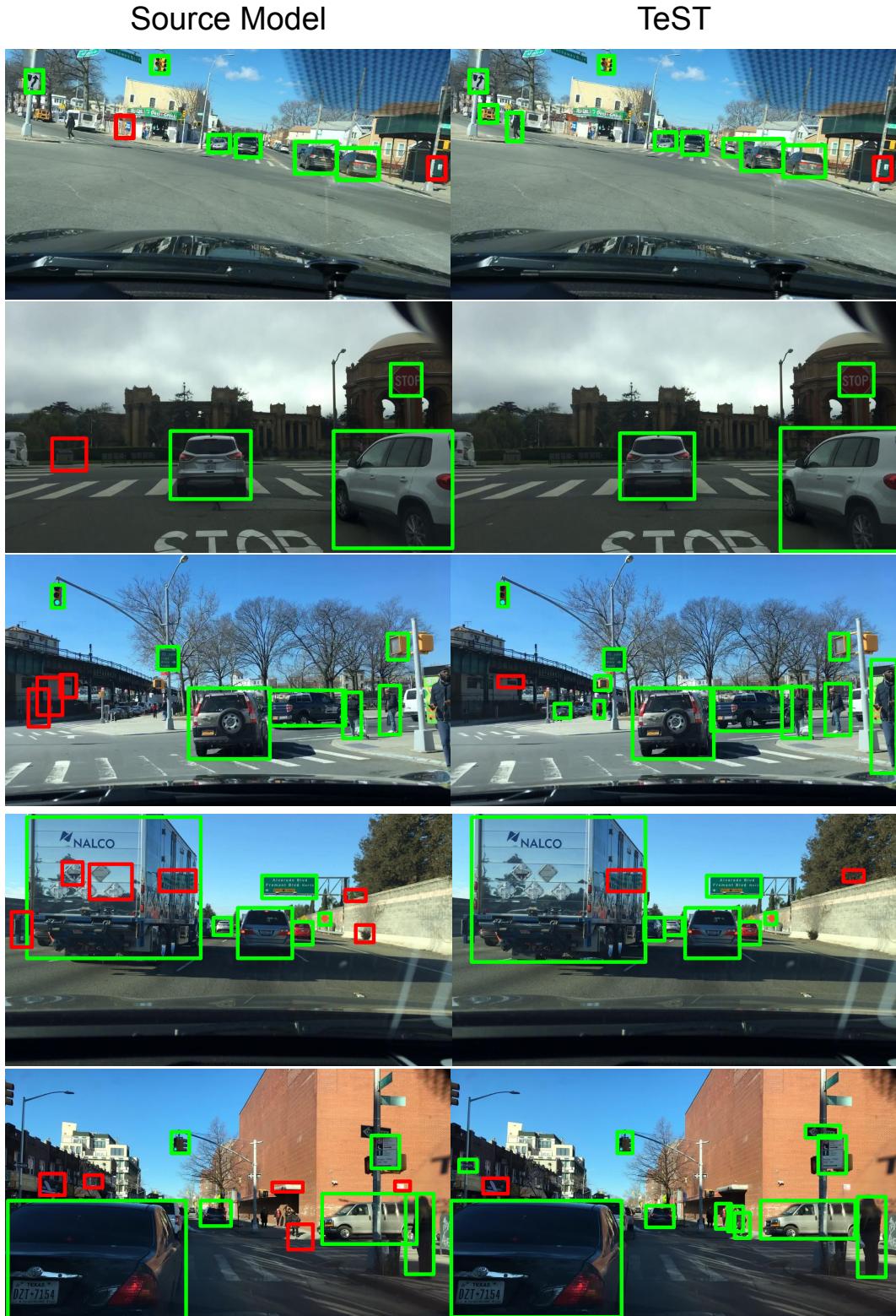
Figure 9: Qualitative results from BDD100k with a Faster RCNN Object Detector [38]. True positives are shown in green rectangles and False positives are shown in red rectangles. We note that: all images are chosen at random without any cherry-picking . We see that the models trained with TeST have fewer false-positives and more true-positives, which strongly suggests that TeST is able to improve the final object detector on the novel dataset.
